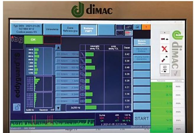
The setup procedure is based on a teach-in process and requires boundary OK and NOK samples available at the operator's place. The setup sequence could be summarized as follows:
