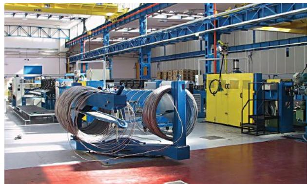
“Wire straightening is performed by a straightener which reciprocates during cut-off (same principle as Flying Shear), so it does not damage the wire as it never twists on the wire in one place. The machines
