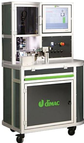
"The Dimac SPC-EVO allows the control of small batches of five to 20 parts in a row, fed in by interchangeable blisters filled off-line. SPC dimensional control and surface inspection are performed on both faces of each piece by two high-resolution digital cameras with bi-telecentric optics and collimated illuminators.
